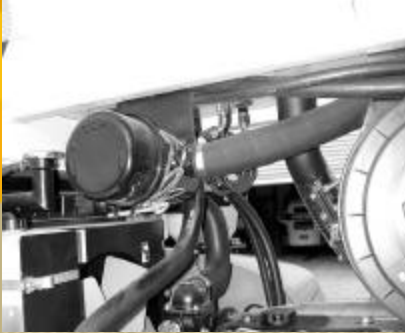
Separate air brake air cleaner
