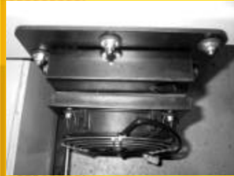
Wet brake oil cooler fitted in the front of the frame
