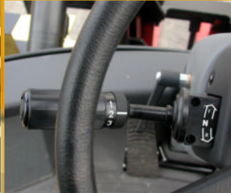
Grip shift gear selector combined with forward/reverse lever
