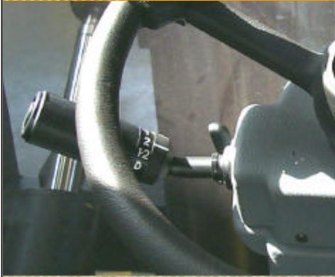
Grip shift gear selector as fitted on trucks with monotrol pedal
