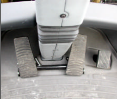
Foot controls on trucks with forward/reverse lever
