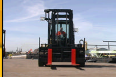
Dual Function Side Shifting Fork Positioner
