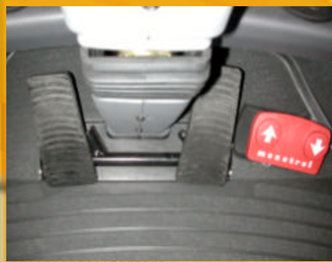
Foot controls on trucks with Monotrol Pedal
